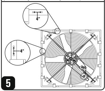
Using marks made in **Step 5** as your guide secure housing to structure using hardware suitable for your structure (not included) and washers compatible with your hardware (not included).
