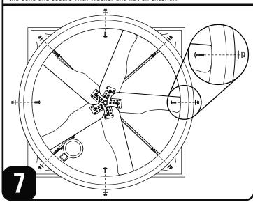
Place guard onto cone flange. Using the guard mounting feet as guides and a 5/16" drill bit, drill holes through cone flange. Secure the guard to the cone using (8) 5/16" carriage bolts and (8) 5/16" nylock flange nuts. Review the Assembly Top View illustration for proper installation. Do not tighten until all have been assembled.
