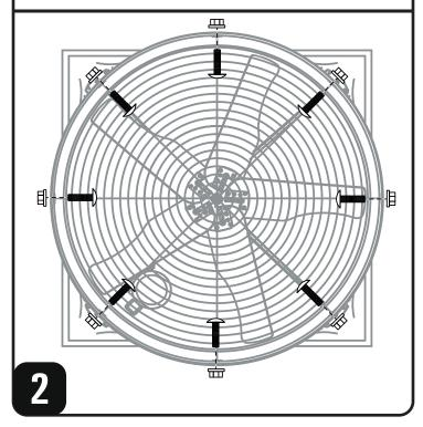
Using the 14 pre-drilled holes in the housing flange attach all (14) shutter clips with a rivet gun using (14) 3/16" rivets and (14) 3/16" backup washers. Review the illustrations below for placement and assembly.
