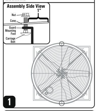
Mark all remaining guard footing locations 1" from venturi edge. Drill holes using 3/8" bit and insert bolts and nuts exactly as you did in step #1. Once all bolts and nuts are installed, go back and tighten each securely.
