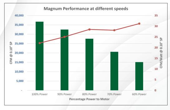
The High Rebate Model is most impressive when you apply certain percentage of power to the motor. When you apply 80% power, you still see an impressive 27,600 CFM at 0.10" SP that is very comparable to our competitor's 100% power, and yet you get an incredible 28.5 CFM/Watt.
