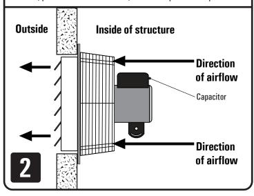
Using appropriate hardware (not provided) for your structure and the weight of your exhaust fan, secure the fan to your structure using the (4) pre-drilled holes on the flange.
