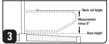
Using the calculated measurement from  $\underline{\text{Step 3}}$  measure and mark a horizontal line on the mounting post, this will be the height of the top of the uppermost twin beam.
