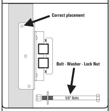
**DO NOT** mount the backer plate with the top mounting hole near the edge of the post or wall edge, see below illustration. To do so can cause wood post failure and any damage resulting from incorrect installation is not covered by warranty.
