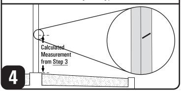
Install twin beams using the mounting brackets and corresponding hardware as chosen for your structure and as illustrated in the following pages.
