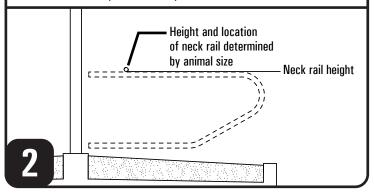
Calculate the measurement from neck rail height to base height and subtract 6" from the measurement.
